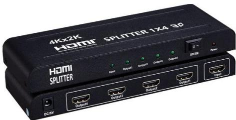
This 1x4 HDMI splitter can connect Set-Top-Box, DVD player, laptop, PS3, PS4, XBOX, HDTV or other HD devices to 4 display devices via HDMI output interfaces and let the 4 display devices show the same picture.
