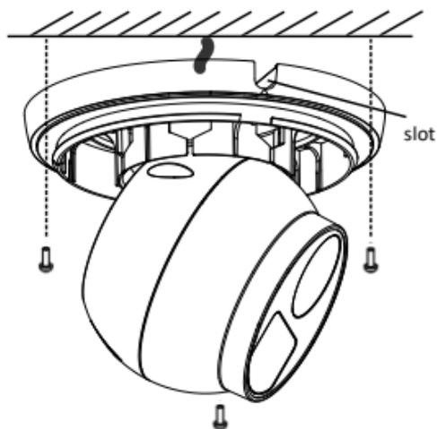
5. Mount your camera. Mount the housing with install mark aligned
