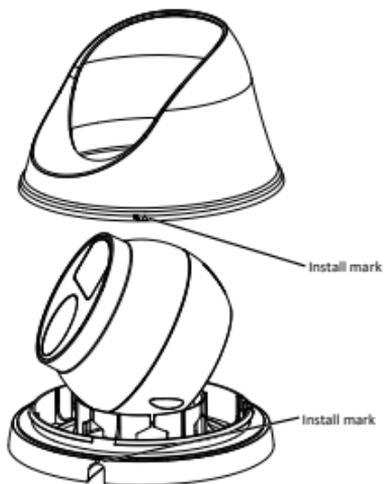
4. Install the base plate and the camera. Connect cable and protect it with waterproof tape and attach dome to ceiling with taping screws.
