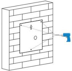
Paste the wall installation sticker on the wall where the equipment needs to be installed. According to the screw hole position on the sticker, use the electric drill to drill the hole with a diameter of 6 and a depth of 25
