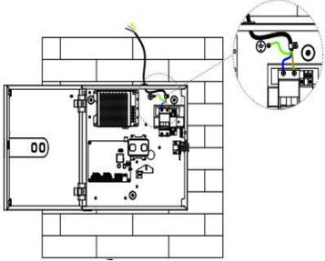
Connect the power cord as shown in the diagram, then it is recommended to use M3X5 screw and wire fastening buckle to fix the power cord to the A092 host machine
