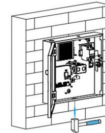
Knock the lead hole with the appropriate tool according to the desired wiring position
