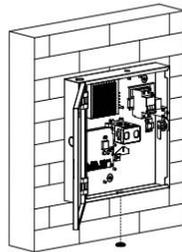
Install silicone pad for lead hole
