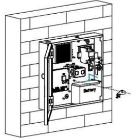
About the installation of the battery: place the battery as shown in the drawing, and use the fixing plate and M3X5 screw to fix.
