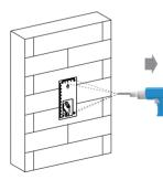
According to the position of the reserved wires on the wall, stick the wall-mounting template vertically to ensure that the wires can come out of the shadow position of template. Drill (6 mm drill bit required) four screw holes with a depth of 25mm in the screw holes of the template.
