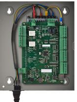
The VS-AXESS-2ETL is a series of powerful and stable access controller, using the logical architecture design. The uplink and downlink adopt TCP/IP and wiegand communicate respectively. Its signal processed with special encryption and can be run offline. Anti-tampering function is also supported.
