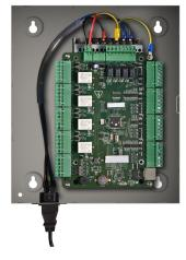
The VS-AXESS-4ETL is a series of powerful and stable access controller, using the logical architecture design. The uplink and downlink adopt TCP/IP and wiegand communicate respectively. Its signal processed with special encryption and can be run offline. Anti-tampering function is also supported.
