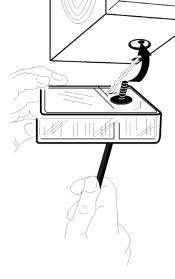
**INSTALL THE SUPPLIED BLACK PLUG-A-HOLE** A) BY SIMPLY SNAPPING INTO THE HOLE.
